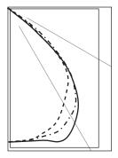
23DS 1T8 lamp with **High Performance** Louver (S90) Efficiency 76.7% Test#13423
